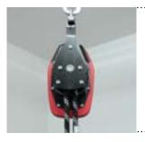
The entire length of the rope was pulled through the device. Now the other end of the rope is roped down.
