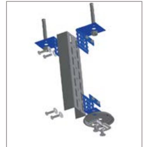
2. Measure the separation height of the suspended ceiling (distance between lower edge of unfinished ceiling and upper edge of suspended ceiling). Cut UA profile **J** to this measurement.
