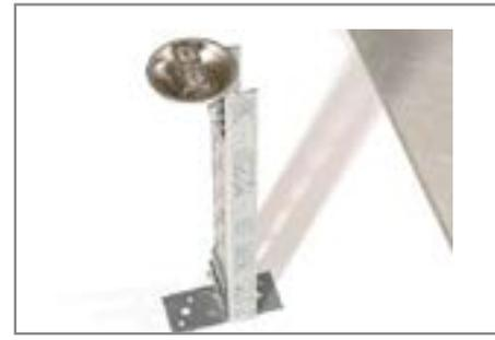
7. Secure absorber **B** to the lower end of the UA profile **J** with 2 x M8 screws **H** and a counterplate **F** and align to the slots so that the absorber **B** is precisely horizontal and 12.5 mm higher than the prepared soffit. (see Figure 3.1.)
