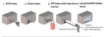
Installation in solid wood/engineered wood
