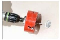
Adjust the ceiling cladding or acoustic plate, calibrate the central point of the absorber B and cut out an opening with a hole cutter.
