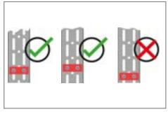
The M8 screws H must not be inserted at the open end of the slots of the UA profile J.
