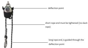
Using the deflection points you can control the descent speed or stop the descent. The longer, unloaded rope end runs through the eye bolts. If you hold on to the longer rope end, you can throttle the descent speed or stop the descent. If you do not use the deflection points, the descent speed will be regulated automatically by a fly wheel brake (speed <2m/sec.).
